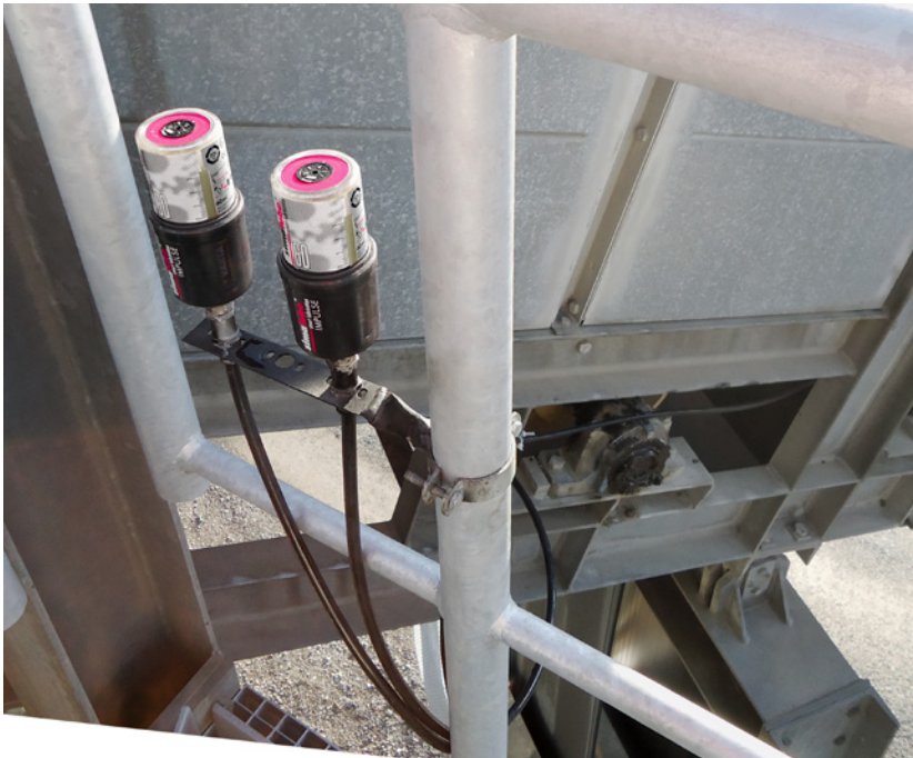
The simalube IMPULSE is mounted in an easily accessible location. With the aid of a long lubrication line, the lubricant can be easily routed to the lubrication point.
