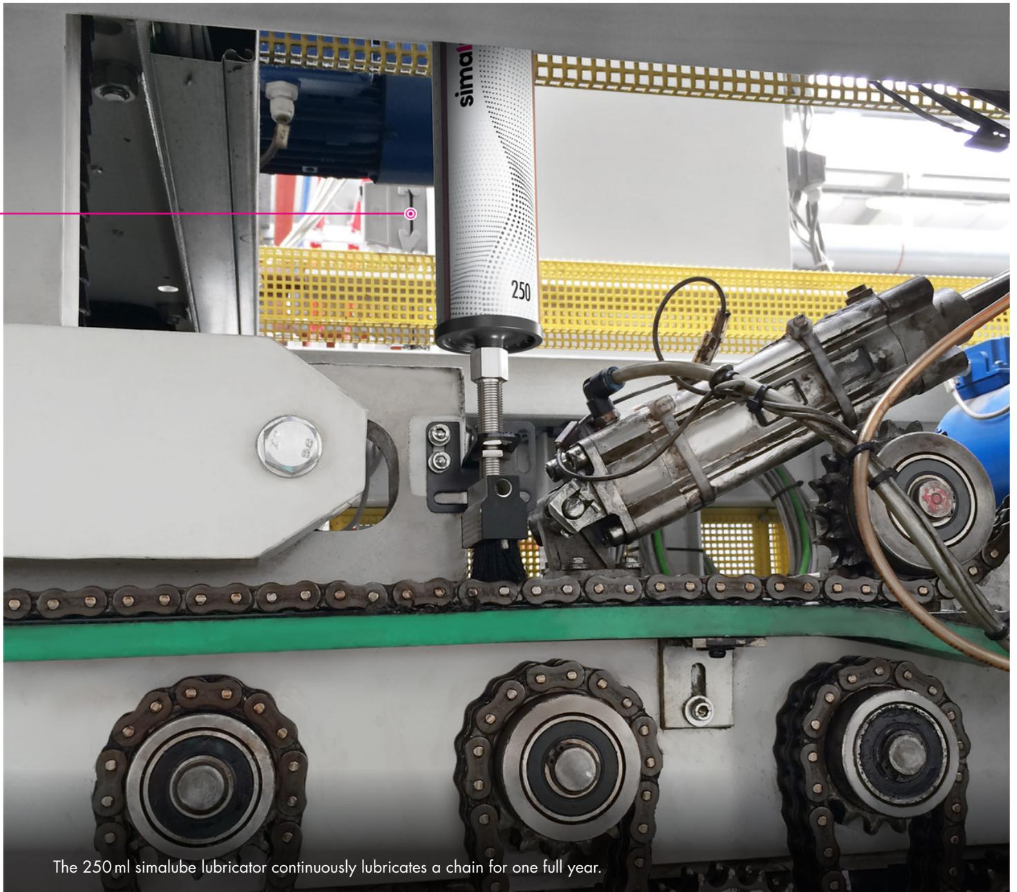
The 250 ml simalube lubricator continuously lubricates a chain for one full year.
