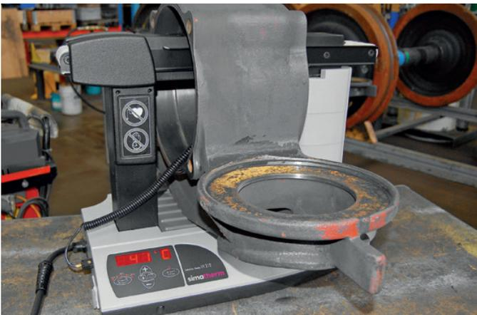
Working on a train wheel-set, the high-performance induction heater IH 210 heats a massive bearing housing to allow a bearing to be inserted.
