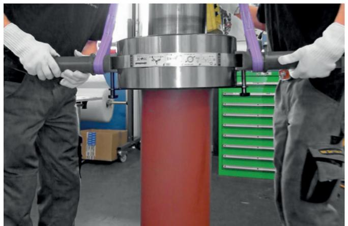
The Bearing Handling Tool BHT allows the heavy, pre-heated roller bearing to be safely lifted and accurately positioned on a turbine shaft.
