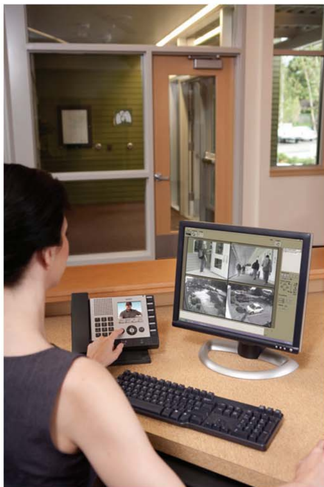
Who's there? A school office receptionist checks with the campus' video intercom before remotely unlocking the door allowing visitors entry into the building. The image in the top left portion of her screen shows a student who is late for class using the school's front door video intercom to gain access to the campus.
