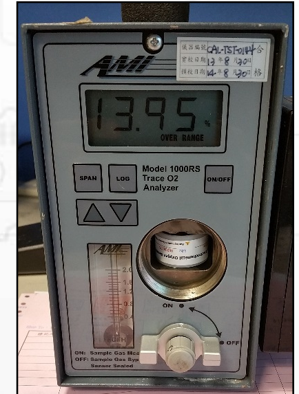
AMI 1000RS with a TO2-1x PPM Replacement Oxygen Sensor Installed. (Tokyo, Japan)
