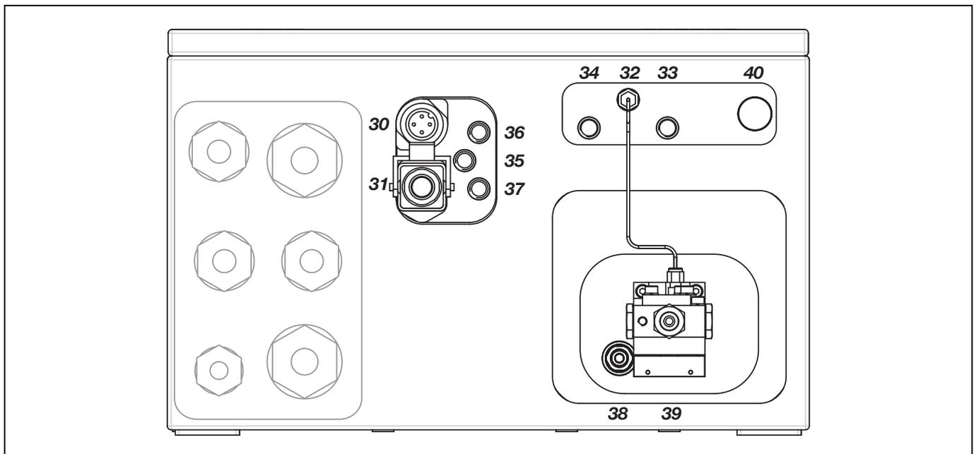
**30** Power supply AC 115 V or 230 V for heating of detector and sample gas inlet (4-pin male plug, connecting cable supplied)
