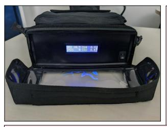
The LFG-30 is a portable gas analyser for the measurement of Methane (CH<sub>4</sub>), Carbon Dioxide (CO<sub>2</sub>), Oxygen (O<sub>2</sub>) and Hydrogen Suplhide (H<sub>2</sub>S). It is ideally suitable for landfill and cogeneration plant applications.
