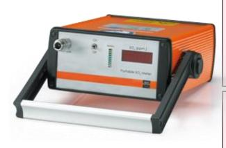
The GMM2000 is a highly specialised device enabling precise measurement of  $SO_2$  in gas mixtures. It is very resistant against contamination and  $SF_6$  decomposition products, and, therefore, a reliable instrument for each revision of circuit breakers.
