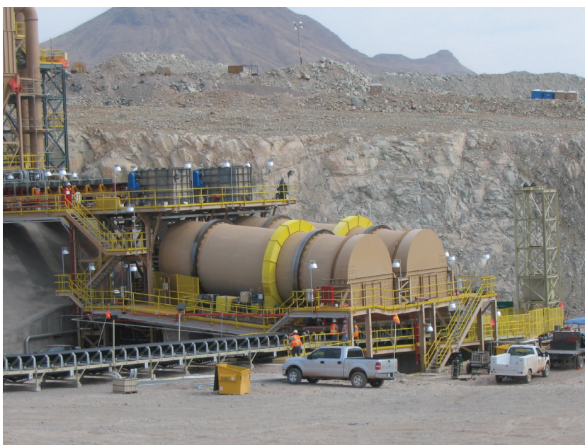
FIGURE 5. Dry agglomeration processes, such as those using drum agglomerators like the one shown here, also use moisture, but significantly less than that used in wet agglomeration processes
