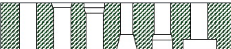
FIGURE 8. Many different die geometries, like the diagrams here, exist, but straight bores are rarely used
