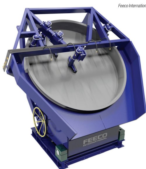
FIGURE 1. This disk pelletizer is an example of a tumble-growth wet agglomeration technology, in which fine particles are wetted with a liquid, usually water
