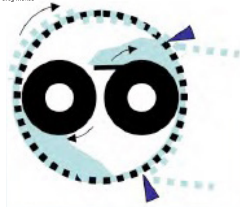
FIGURE 7. In a ring die mill, powder is fed into the interior of a cylinder and rollers push the material out through holes in the cylinder
