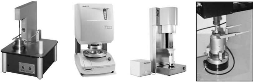
**Figure 4.4. Automated testers; from left to right: Schulze and Brookfield Engineering annular ring shear testers; Freeman Technology and E&G Associates (Peschl) torsional testers.**
