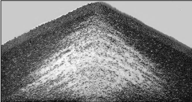
**Figure 8.6. Sifting segregation after formation of a pile.**
