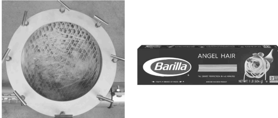
Figure 7.40. Angel hair from pneumatic conveying line (left) and my local grocery store (right).
