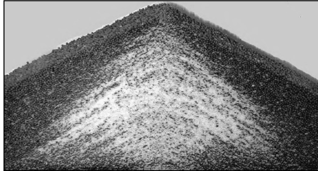
Figure 7.2. Sifting segregation after formation of a pile.
