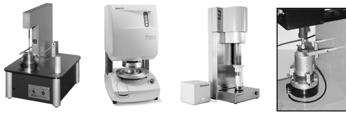
Figure 4.4. Automated testers; left to right: Schulze and Brookfield Engineering annular ring shear testers, Freeman Technology and E&G Associates (Peschl) torsional testers.
