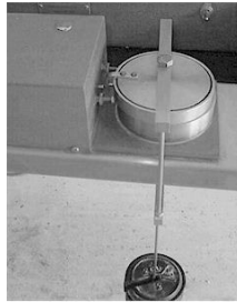
Figure 4.3. Jenike direct shear cell tester.
