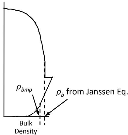
**Figure 3. Comparison of  $\rho_{bmp}$  and the bulk density at the cylinder-hopper junction.**
