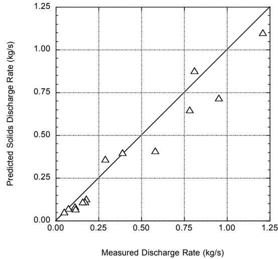
**Figure 4. Comparison of measured and predicted solids discharge rates.**
