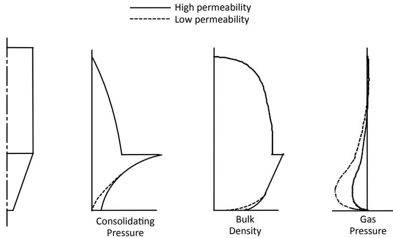
**Figure 2. Consolidating pressure, bulk density, and gas pressure profiles for coarse (high permeability) and fine (low permeability) powders.**
