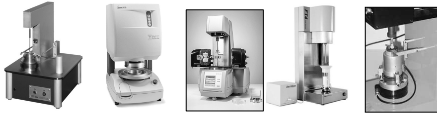
Figure 4.4. Automated testers; left to right: Schulze, Brookfield Engineering and Anton-Paar annular ring shear testers, Freeman Technology and E&G Associates (Peschl) torsional testers.
