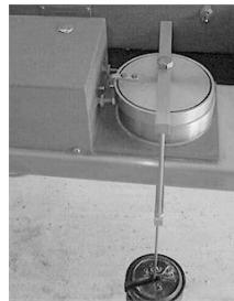
Figure 4.3. Jenike direct shear cell tester.
