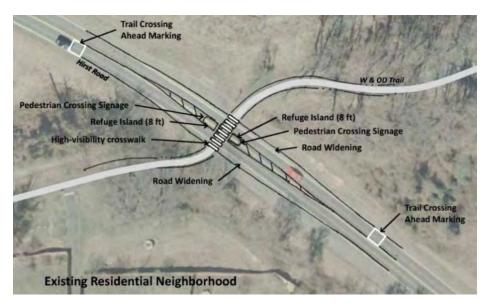
Figure 10 – Recommended W&OD Trail Modifications at Hirst Road (Purcellville's Transportation Plan)
