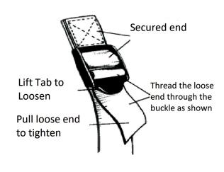
Some of the straps may have to be adjusted for proper fit depending on the user and the vehicle.
