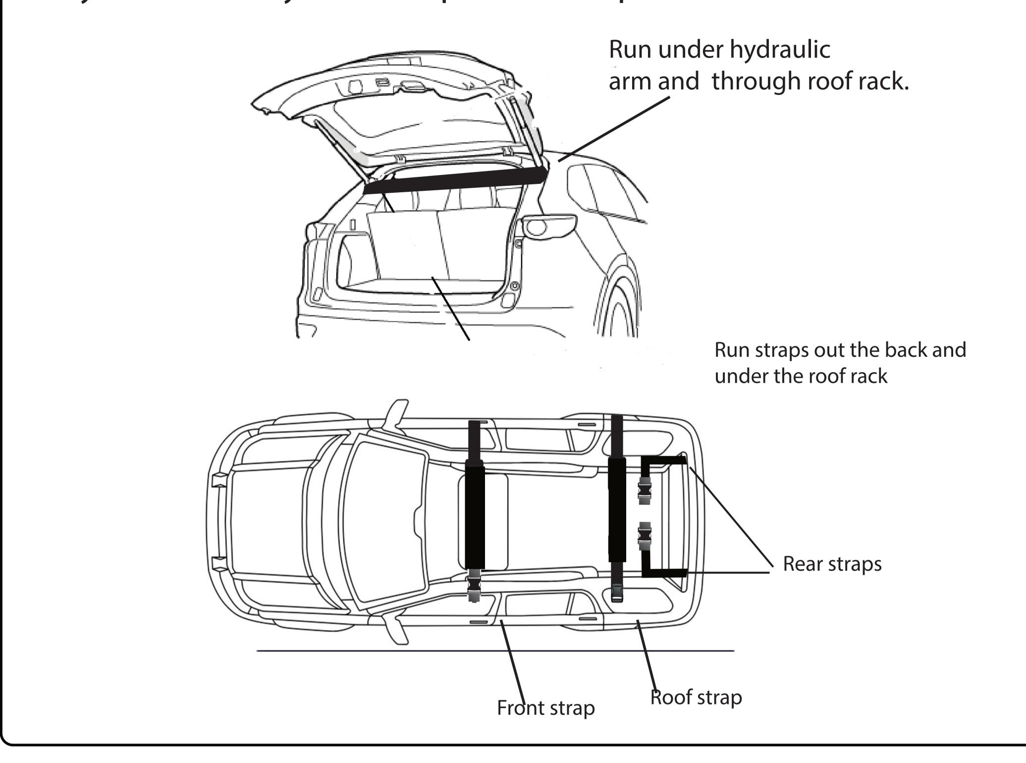
**Step 6 -** Connect the two carabiners on top of the vehicle and adjust the straps.
