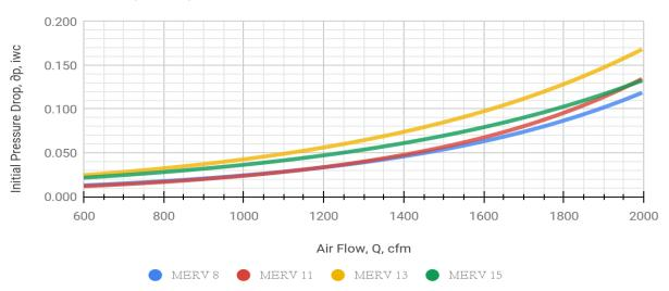
represents the performance data for our 21" wide furnace filter cabinet prototype utilizing 3 - 20"x25"x2" Columbus Industries filters.
