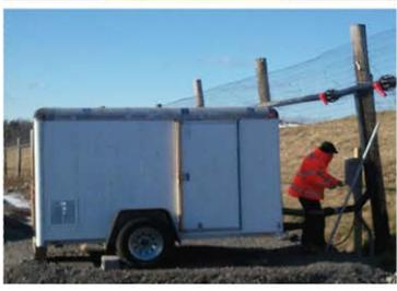
Connet unit to Power: 460/3/60, 20.5 Amps Service 4 wire 10 Gauge SO
