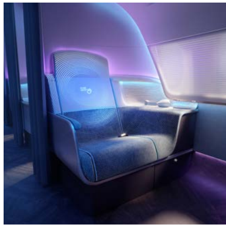
Using reactive thermochromic or photochromic ink technologies, seats and surfaces that are thoroughly cleaned temporarily display the Pure Skies logo to reassure boarding passengers.
