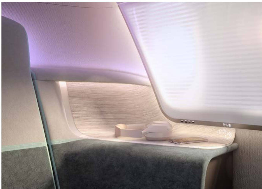
Advanced printing and finishing techniques enable replacement of some carpet and textile applications with easier-to-clean plastics that offer a high-end look, such as on this seat-side table in business class. (above)
