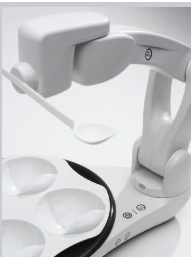
The commercial version of Obi on sale now consists of 33 parts. PTI Engineered Plastics in Michigan made the aluminum tools and molded all of the plastics components.
