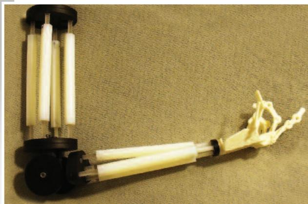
**Left: Nonspec's patented pylon system adjusts for height, width and angular adjustment to perfect a patient's gait while they are wearing the prosthetic. Above is an early version of Nonspec's prosthetic arm and robotic hand.** Photos courtesy of Nonspec Inc.
