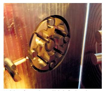
Made just a few months ago, this is the first low-volume injection mold insert that Nonspec had produced to test the mold design of one of its lower limb plates. Courtesy of Nonspec Inc.
