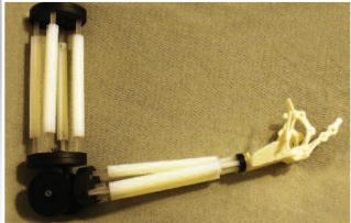
Left: Nonspec's patented pylon system adjusts for height, width and angular adjustment to perfect a patient's gait while they are wearing the prosthetic. Above is an early version of Nonspec's prosthetic arm and robotic hand. Photos courtesy of Nonspec Inc.
