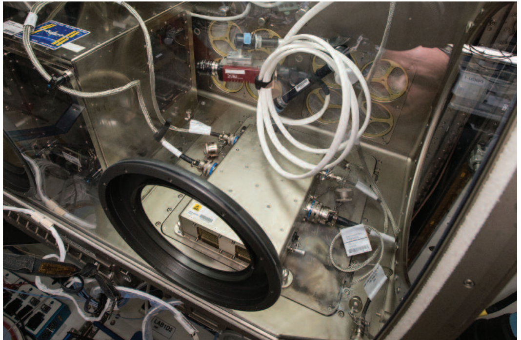
The International Space Station's 3D printer is shown configured in the Microgravity Science Glovebox. Testing this on the station was the first step toward creating a working machine shop in space. This capability may decrease cost and risk on the station, and will be critical when space explorers venture far from Earth and will create an on-demand supply chain for needed tools and parts. Courtesy of NASA
