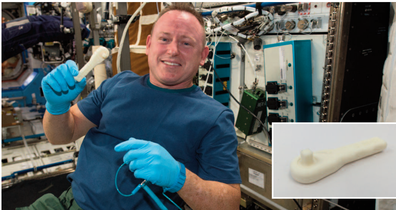
Pictured here in December 2014, NASA astronaut Barry (Butch) Wilmore holds a 3D printed ratchet wrench from the new 3D printer aboard the International Space Station. The printer completed the first phase of a NASA technology demonstration by printing a tool with a design file that was transmitted from the ground to the printer. (Inset) Ratchet print for NASA made as a demonstration of a tool. Images courtesy of NASA
