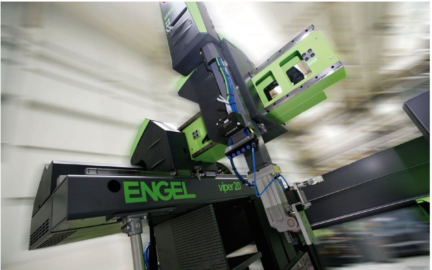
Engel’s viper linear robots now come with a longer range than before, enabling longer take-off strokes.
