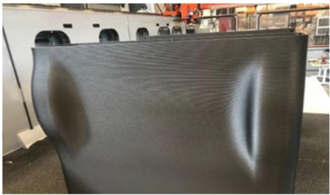
Base of the HAT 2.0's water module, as printed from carbon fiber-filled ABS on the Thermwood LSAM (left). HAT 2.0's final water tank, which can hold 3,615 liters of fluid. Courtesy of Launch Forth
