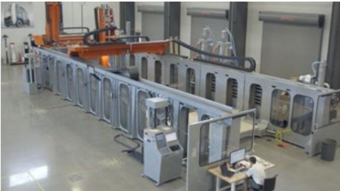
**Thermwood LSAM 3D printer in LM Industries' Knoxville, Tenn., microfactory.** Courtesy of Launch Forth
