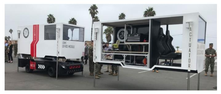
MLV module platform, in the midst of transition from the administrative module (left) to construction module (right), at Camp Pendleton, Calif. Courtesy of Launch Forth
