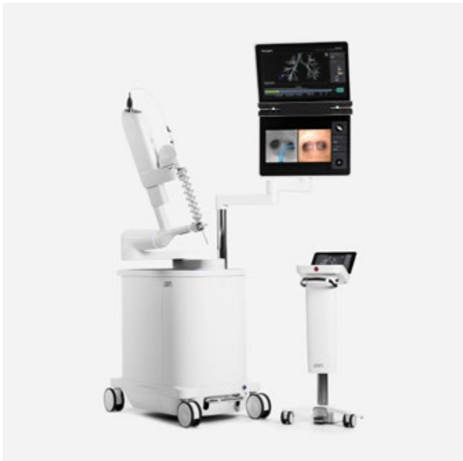
Intuitive Surgical Inc. won gold and best in show for its well-considered execution of a robotic device to perform minimally invasive biopsies deep in the lung. Courtesy of IDSA
