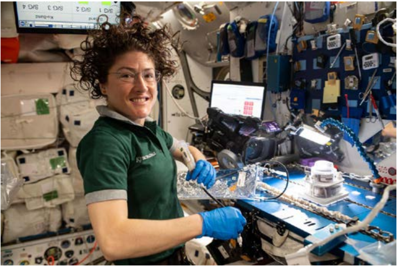
NASA astronaut Christina Koch works on space botany research using the Veggie POND gear to cultivate and harvest lettuce and mizuna greens for consumption on the International Space Station and analysis on Earth. Courtesy of NASA
