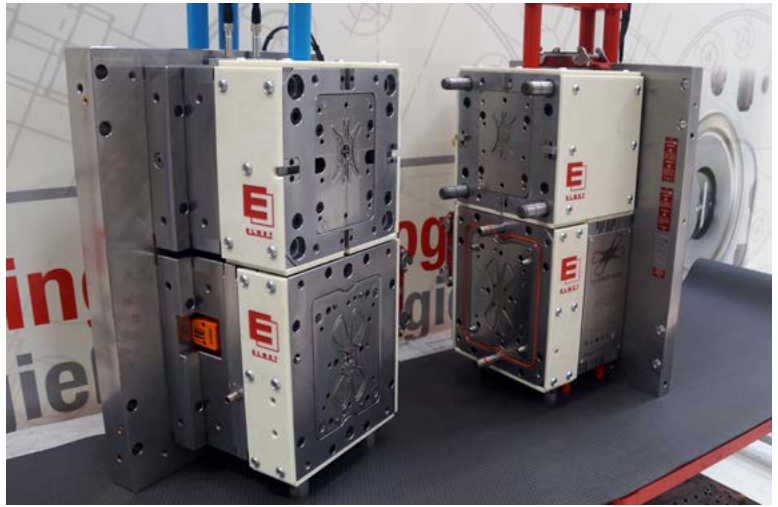
Austrian tool maker Elmet Elastomere GmbH made the mold needed to make the winning, two-component "Butterfly" cellphone holder using flexible LSR and rigid polycarbonate.
