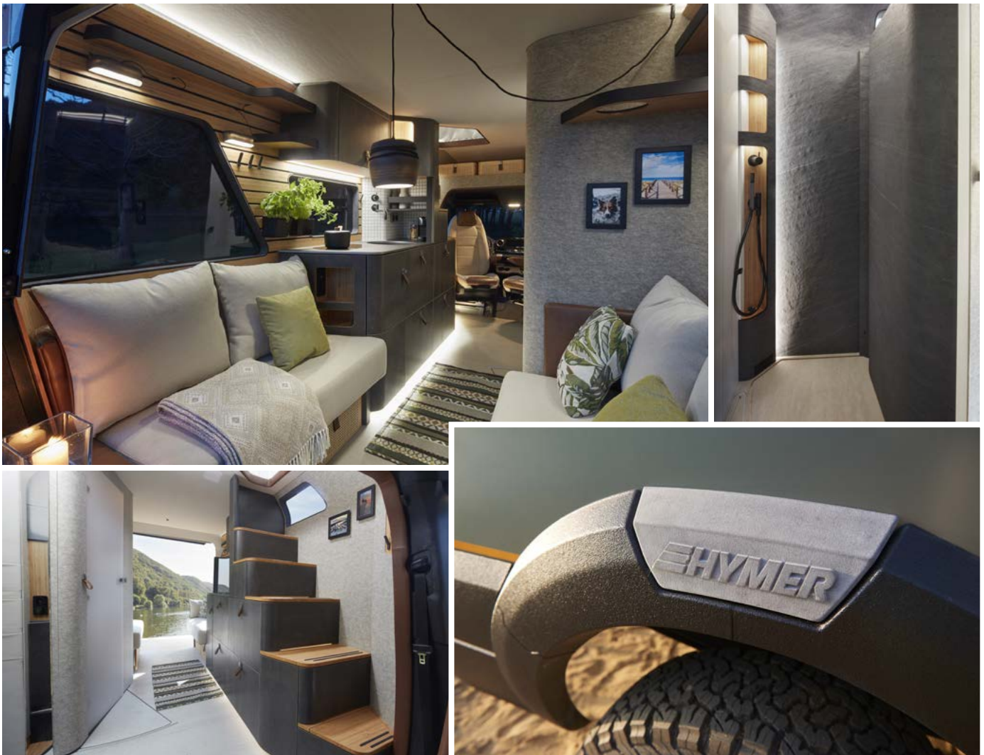
Many of the camper’s living areas are multifunctional, including a wet/dry bathroom and a living room that can double as an office. (top-left) Hymer applied BASF’s Veneo Slate, a pliable surfacing material with razor-thin, natural-stone facing, to the camper’s bathroom walls. (top-right) Using many “tiny home” concepts, the van offers storage underneath the LED-illuminated staircase. (bottom-left) The vehicle includes more than 100 3D-printed components, including this wheel-arch cladding. (bottom-right)
