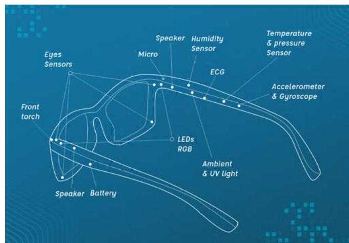
Ellcie Healthy embeds 15 sensors in their eyeglass frames, made of nylon 12, that can detect a number of different factors, including nodding, blinking, and even yawning. Courtesy of Ellcie Healthy
