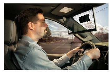
Bosch noted how it leveraged AI to develop the Virtual Visor, a vehicle sun visor that blocks only the areas where the sun blinds the eyes, while allowing an otherwise unobstructed view. Courtesy of Bosch
