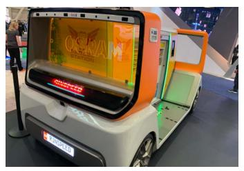
Switzerland's Rinspeed AG displayed its MetroSnap modular concept vehicle on the CES stand of its partner, lighting maker Osram GmbH. The body can be easily swapped out on the chassis, enabling various end-use functions, from moving people to dispensing packages or food. Photo by Robert Grace
