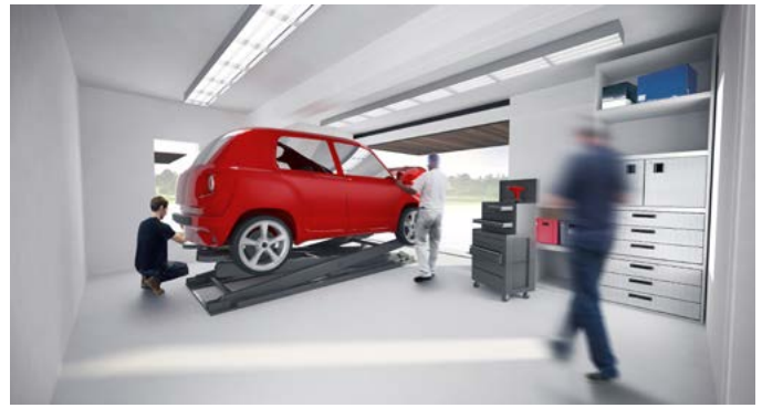
Gazelle Tech's modular microfactories ship in six 20'-long by 8'-wide shipping containers and cover about 1,075 square feet when assembled into an office and workshop area. (left) The microfactories are spacious enough to allow for assembly of the entire car. (right) Courtesy of Gazelle Tech
