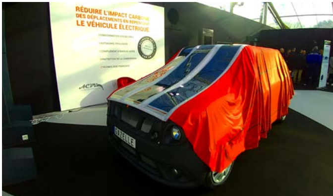
Gazelle Tech displayed this prototype solar cover at a recent Paris auto show. It rolls upward from behind the rear bumper to cover the car and potentially provide additional driving range by charging the battery from the cover's flexible solar panels. Courtesy of Gazelle Tech
