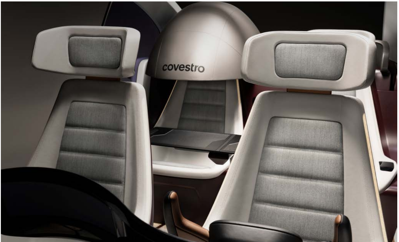
The back seat features a movable privacy dome with sound-absorbing acoustic materials to provide an oasis of peace and quiet. Courtesy of Covestro
