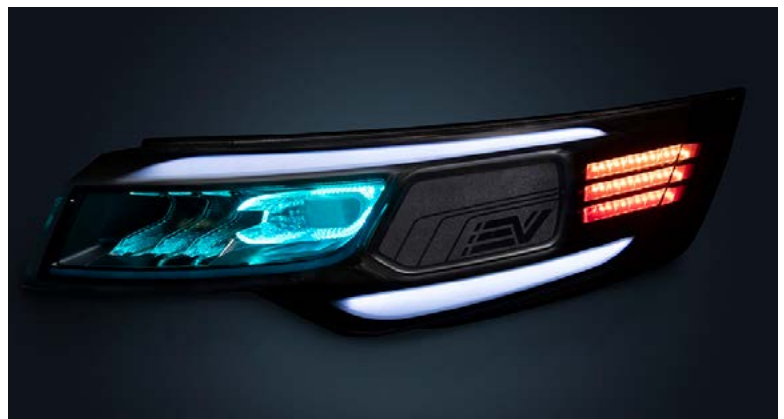
Covestro's multifunctional, mono-material headlamp design leverages thermally conductive PC to eliminate heavy, costly aluminum heat sinks, while using multishot injection molding and in-mold assembly to simplify production and lower cost. Courtesy of Covestro
