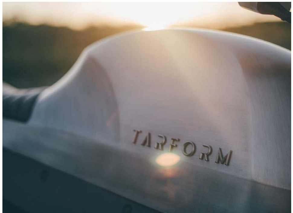
Instead of gluing logo letters to the side of the bike, Tarform 3D prints them and mechanically attaches each one. Courtesy of Tarform
