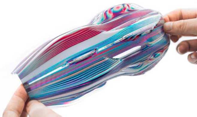
Two designers at MIT used multimaterial voxel 3D printing and a computational workflow they devised to create Illusory Material, which enables designers to realize and manipulate color and texture in physical items. Courtesy of IDSA
