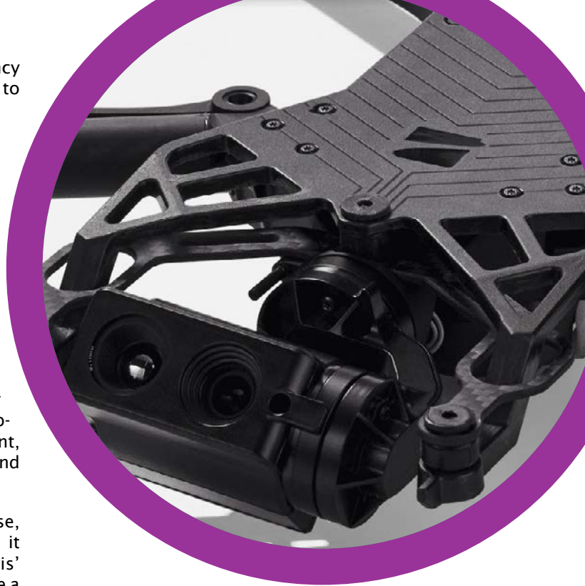
Skydio says that 3D printing this upper plate using Arris' composite technology lets it consolidate 17 parts into one and reduce weight 25 percent. (above) Courtesy of Skydio
