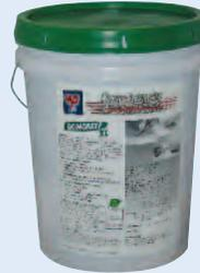
Leveling Compound is supplied in 50-lb pails and consists of specially formulated components. Just add water, mix and compound is ready for troweling. It will not shrink as it dries and can be featheredged. One drum covers 50 square feet of surface in 1/8" thickness. Compound adheres to most surfaces; wood, concrete, steel, marble, etc. No primer required.
