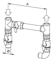
In realising the dryer, particular measures have been taken in order to limit the vibration which could occur during the operation. Therefore we recommend to use connecting pipes able to insulate the dryer from possible vibrations originating from the line (flexible hoses, vibration damping fittings, etc.).
