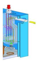
The condensate is discharged from the heat exchanger by an electric time drain that is controlled from the DMC15 controller. Drain open times are adjustable between 1 to 10 seconds and the closed time is adjustable between 1 to 10 minutes. A manual push to test makes checking the condensate drain operation quick and simple.
