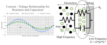
The rate of chemical processes sets limits on the frequency that each process can follow, so the voltage-current data is collected over a wide range of frequencies, allowing the various processes to be measured independently. The voltage-current data is modeled as an electrical circuit of resistors, capacitors, and other elements, which is fit to the data using non-linear least squares. Each element of the circuit models a particular chemical process as shown above.
