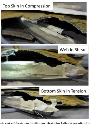
This set of features indicates that the failure resulted in an overload of the structure that likely was the result of the accident.
