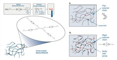
The relative rates of chain lengthening and crosslinking over time is controlled by chemicals called hardeners and possibly accelerators and by the temperature profile of the cure cycle. The viscosity of the resin first decreases and then increases over time as shown by the figure below. Pressure is applied when the viscosity is low to consolidate the composite and remove air bubbles.
