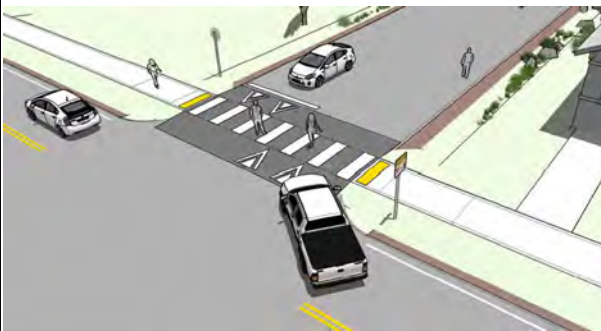
Use raised crosswalks for pedestrian or aspirational pedestrian areas (e.g., Town Green municipal campus, Lancaster Center, and Main St., South Lancaster by the bridge).
