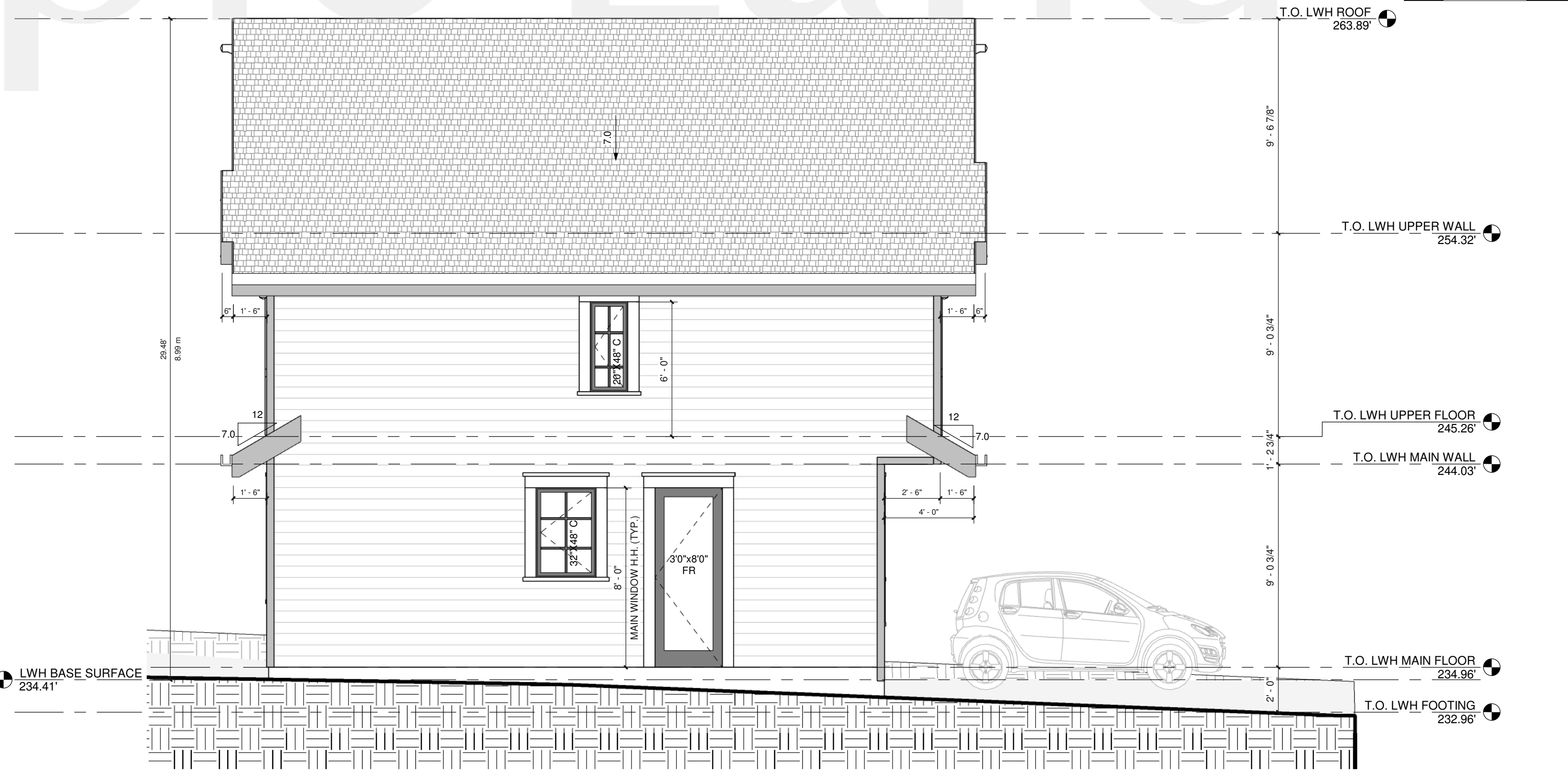
2 LWH SIDE ELEVATION (W) 1/4" = 1'-0"
