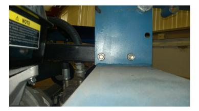
Caution! The log splitter frame is heavy and awkward. It is mandatory to have two people to lift and stabilize the main frame assembly while securing to the axle frame assembly!
