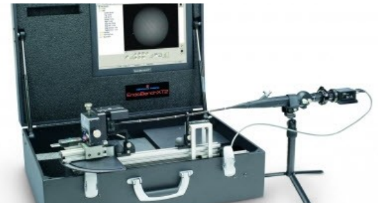
Flexible scope testing using EndoBench XT™
